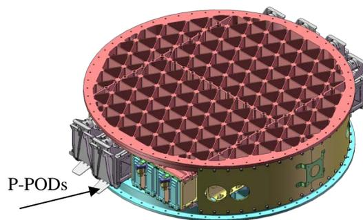
**Figure 3.4** The Loadpath Engineering Cubestack Wafer can accommodate up to eight P-PODs or equivalent dispensers.
