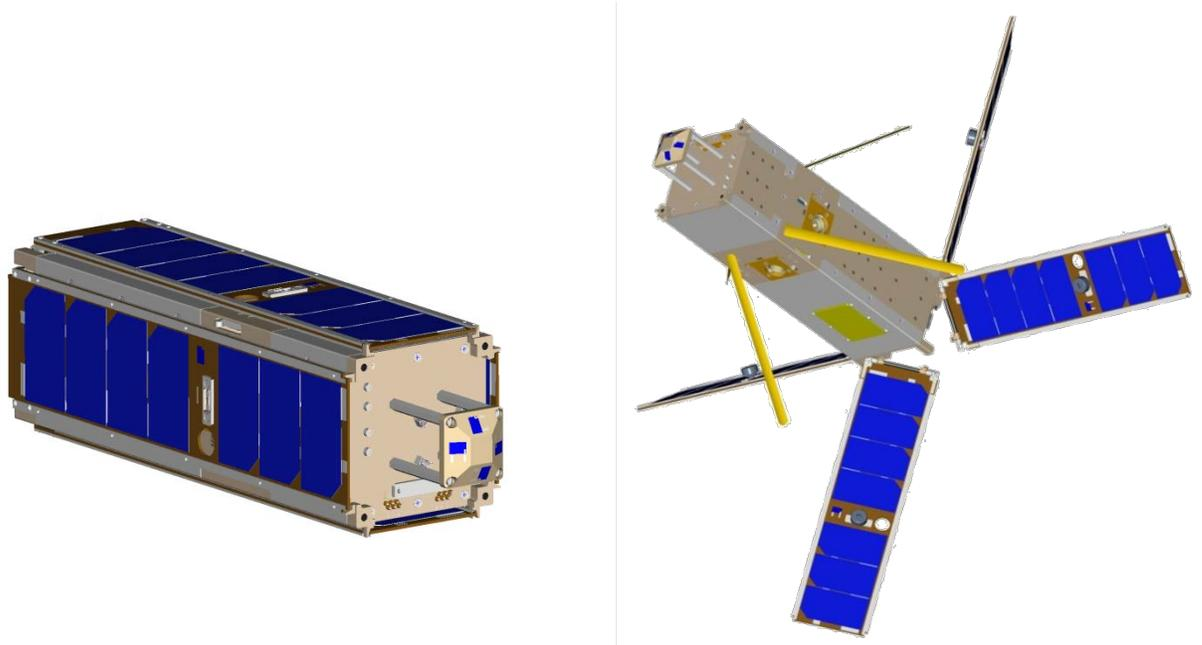
**Figure 4.1** Stowed (left) and deployed (right) operational configurations of the ORS Tech space vehicle.
