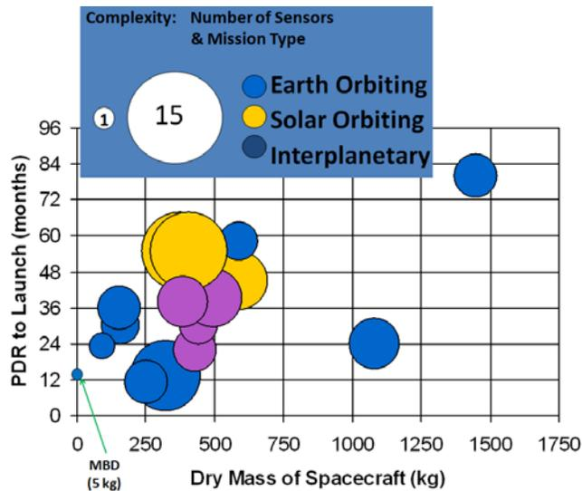
Figure 2.1 Comparison of a few satellites built by the Johns Hopkins University Applied Physics Laboratory contrasting size, complexity, and time to launch
