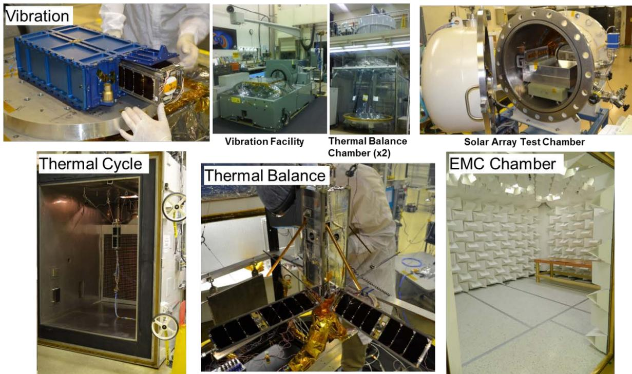
**Figure 4.2** Complete testing of the ORS Tech 1 & 2 space vehicles was performed to ensure design integrity, workmanship, functionality, and operation across all launch environments and mission phases.
