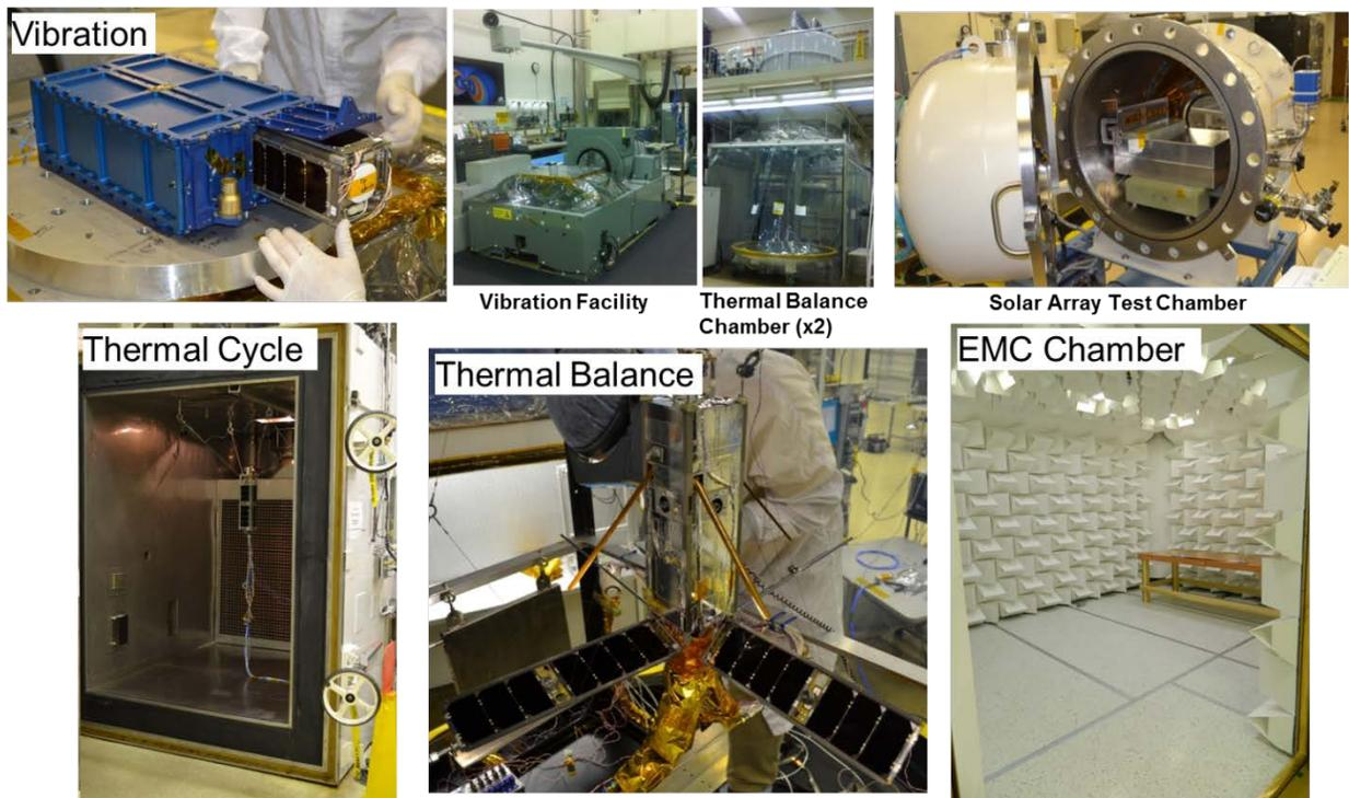
**Figure 4.2** Complete testing of the ORS Tech 1 & 2 space vehicles was performed to ensure design integrity, workmanship, functionality, and operation across all launch environments and mission phases.
