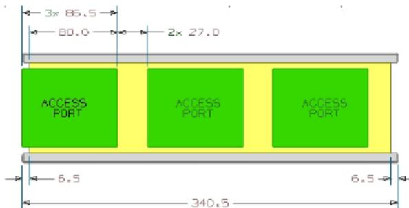
**Figure 3.2** Side view of a 3U CubeSat
