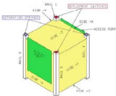
Figure 3.1 Isometric view of a 1U CubeSat
