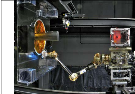
Figure 17: FRENDA arm at NRL equipped with Marmon ring grasping tool has been successfully demonstrated many times in a variety of configurations and lighting conditions. (NRL image)
