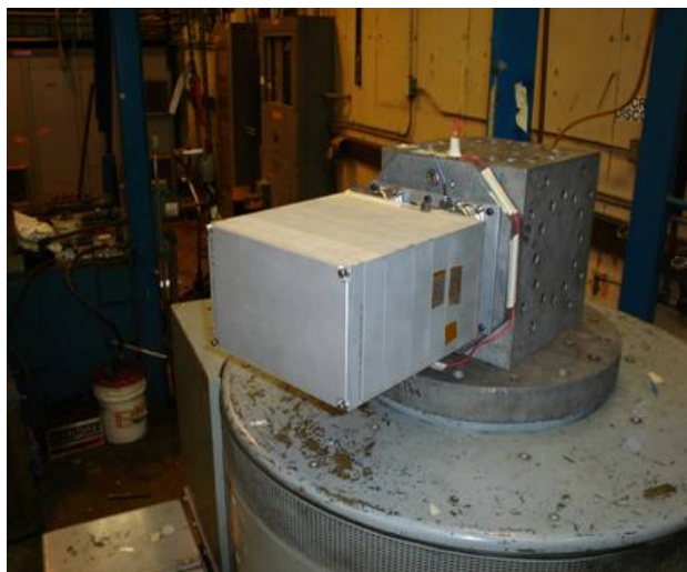
Figure 3 - X-Axis Random Vibration Test
