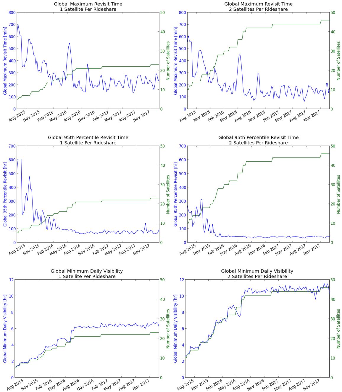
Figure 3: Coverage metrics vs. time, building up a rideshare-initiated constellation using the rideshare manifest in Table 1. The left column shows metrics using 1 satellite per rideshare, and the right column shows metrics using 2 satellites per rideshare.
