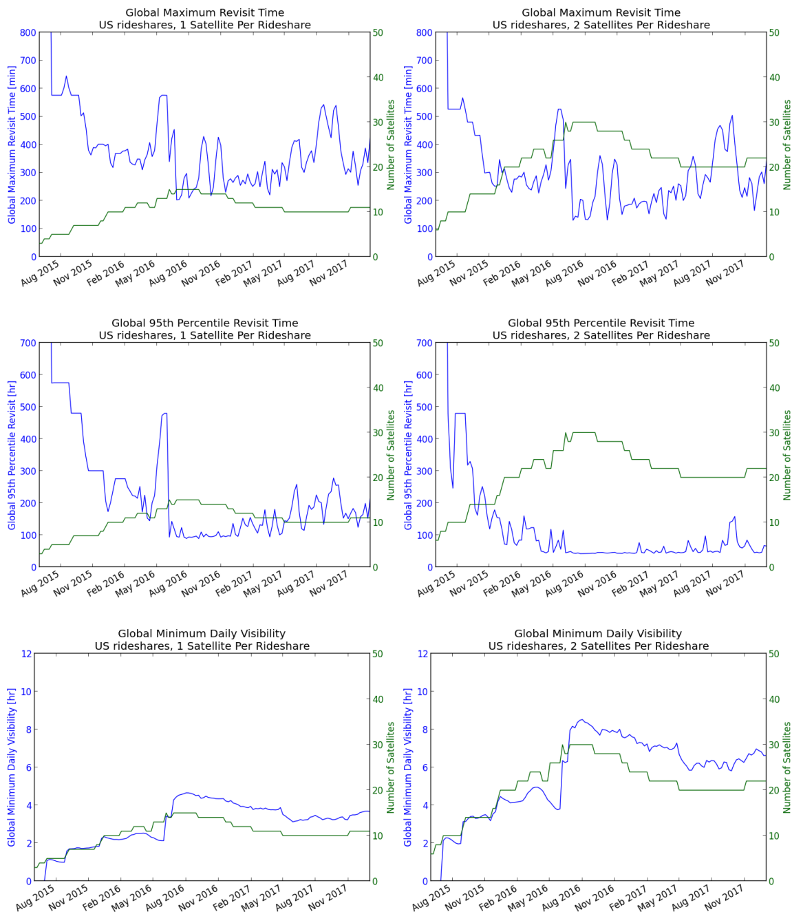
Figure 4: Coverage metrics versus time for a rideshare-initiated constellation that uses only US launch vehicles and assumes that ISS-deployed CubeSats leave the constellation after 1 year due to atmospheric reentry. The left column shows metrics using 1 satellite per rideshare, and the right column shows metrics using 2 satellites per rideshare.
