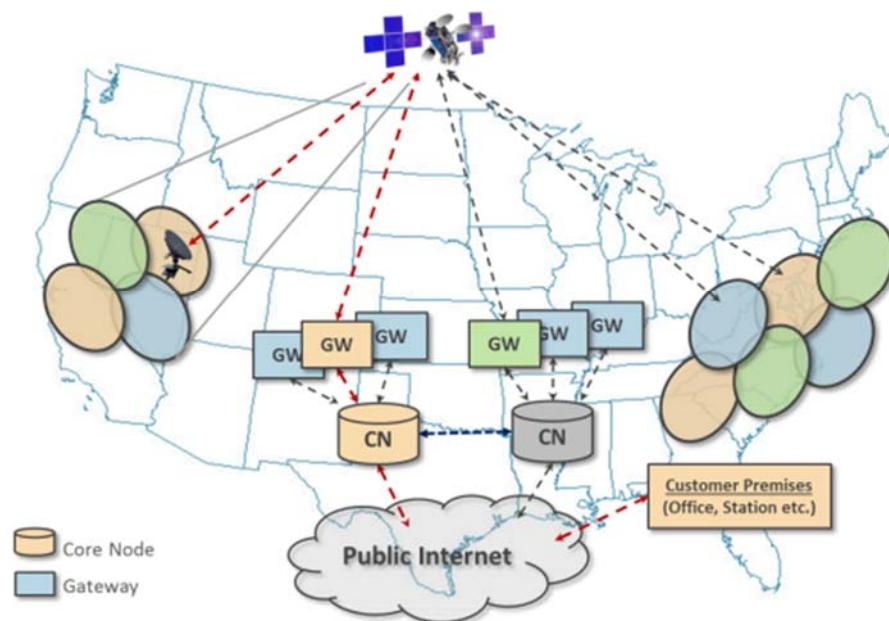
**Exhibit 3: High Capacity Satellite Beam Architecture**
