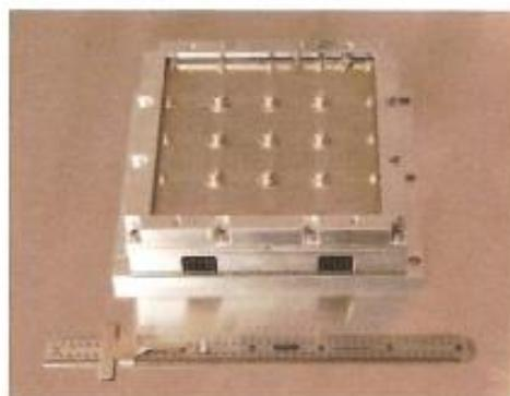
**Exhibit 7:** Photographs of the iMESA instrument flown on the International Space Station during 2009-2001 onboard the MISSE7 platform. The ion entrance slits are on top of the instrument.
