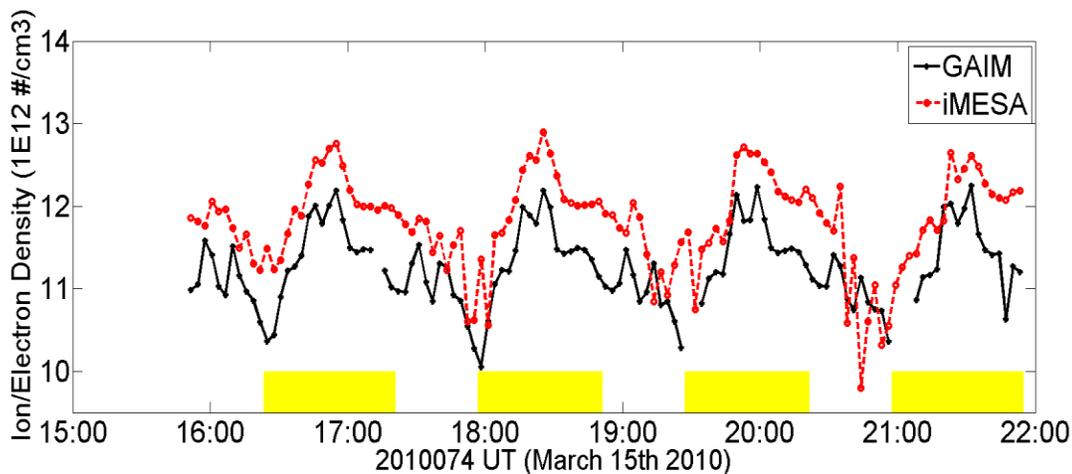
**Exhibit 11:** MISSE-7 iMESA plasma density data plotted with GAIM derived density data interpolated onto the ISS/MISSE-7 orbital track over four orbital time periods. Sunlit periods are shown by the yellow bars.
