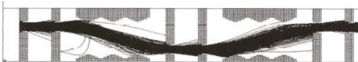
**Exhibit 8:** Cross-section of iMESA instrument detector head, consisting of 3 sets of grounded collimating plates (left, center, and right) and 2 biased electrostatic deflection chambers (with scalloped edges and between the sets of vertical collimating plates). Charged particles enter at the left and exit at the right.
