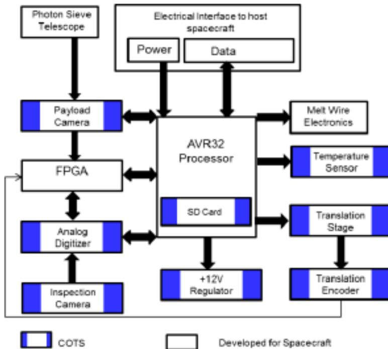
**Exhibit 6:** Peregrine payload electronics block diagram. Arrows indicate C&C signal flow.
