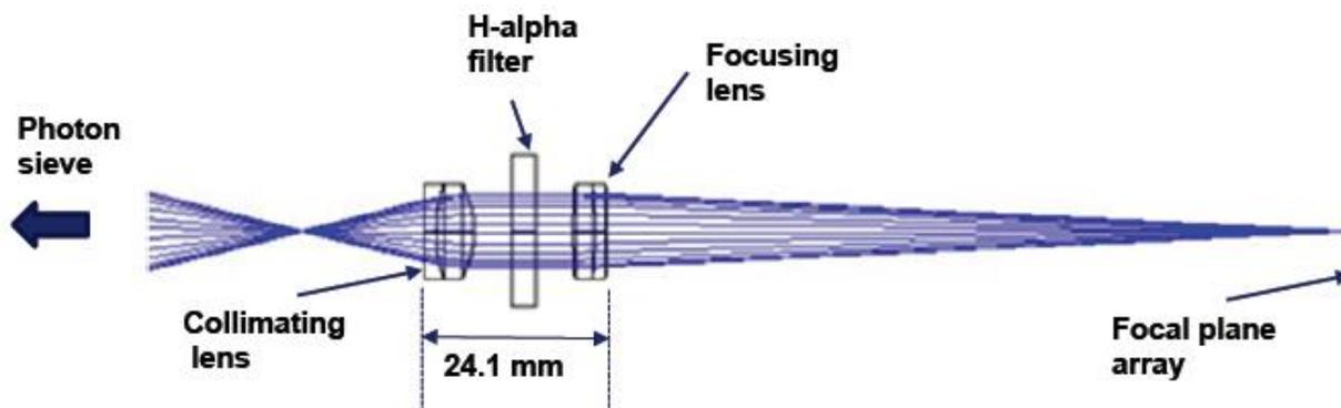
**Exhibit 3:** Peregrine telescope schematic. Focused light from the photon sieve to the left (not shown) passes through two lenses and filter. The collimated beam is approximately 10 mm in diameter, and the final focal distance from the second lens to the camera focal plane is about 100 mm. The three fold mirrors after the final lens are not shown.
