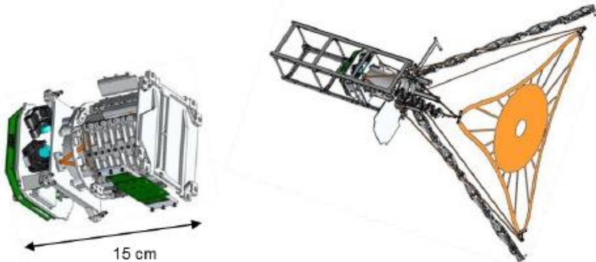
**Exhibit 1:** Stowed (1.5U) and deployed Peregrine payload schematics.
