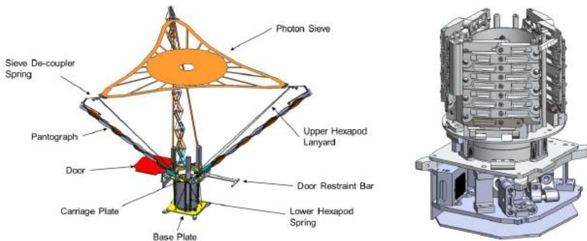
**Exhibit 4:** Left CAD drawing illustrates the double hexapod deployment structure and final positioning of the membrane. Right CAD drawing shows the stowed configuration of the pantographs symmetrically surrounding the central tube which houses the folded photon sieve. The secondary optics and CCD camera are located on the lower platform which is pinned and bolted to the base plate of the deployment assembly.
