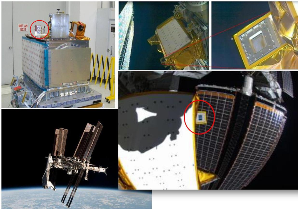
**Exhibit 13:** Clockwise from top left: The Canary instrument integrated on the STP-H3 ExPA pallet. ExPA pallet and Canary experiment mounted on the port-side truss of the ISS. Canary instrument photographed by astronaut whose shadow is visible on the left of the photograph. The STS position with respect to the Canary boresight.
