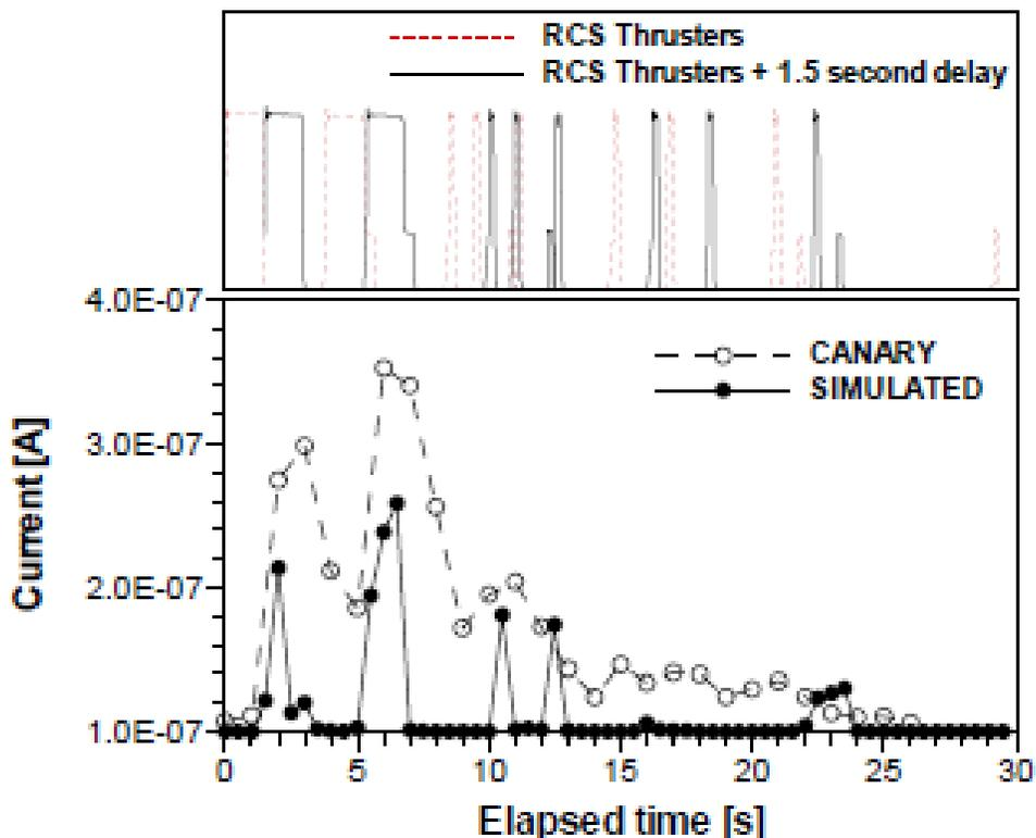
**Exhibit 14:** Comparison of Canary and simulated ion current as a function of time during the 30 May 2011 Space Shuttle Endeavour NH2 maneuver. RCS thruster chamber pressure as a function of time is also shown.
