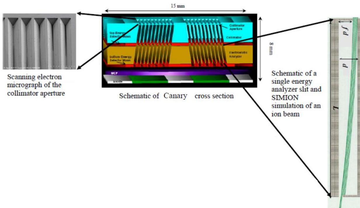
**Exhibit 12:** Important features of the Canary ESA instrument. Space plasma ions enter through the collimator at the top of the sensor head, pass through the ESA plates, MCP, and collect at the anode at the bottom.
