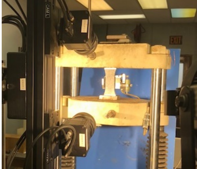
Exhibit 6. DIC measurement performed on an aluminum coupon during tensile testing.
