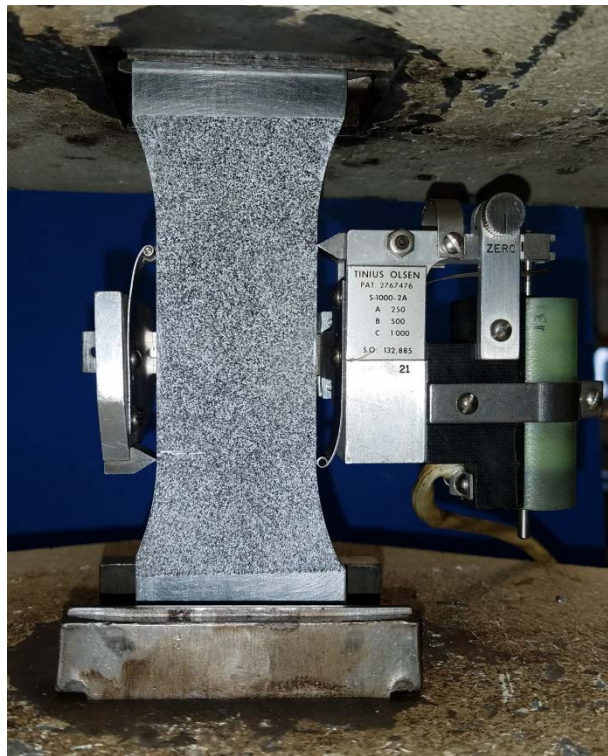
Exhibit 7. Aluminum coupon installed in tensile testing machine with 2 inch clip gage attached and surface speckled pattern for DIC.
