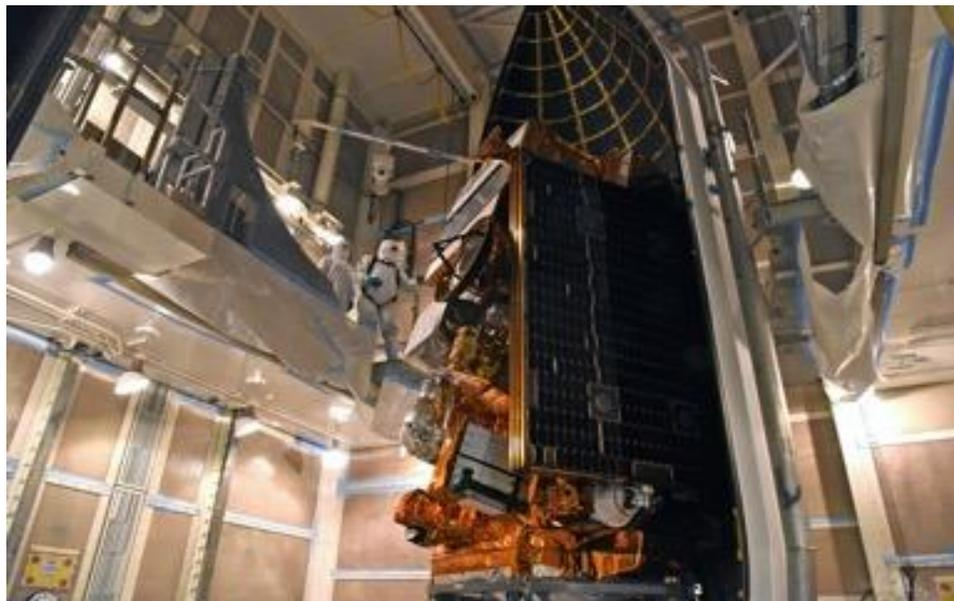
**Exhibit 11.** JPSS-1 Satellite During Delta II Launch Vehicle Fairing Installation.<sup>4</sup>
