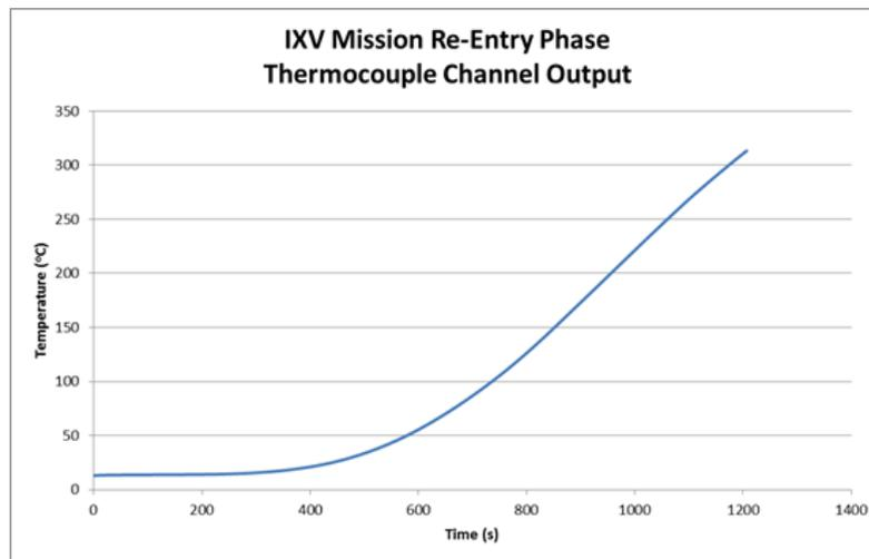
Figure 7: Thermocouple sensor data from IXV Mission
