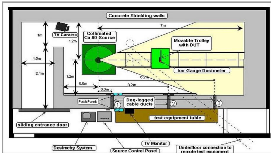
Figure 4: Cobalt 60 gamma radiation facility (Courtesy of ESA)
