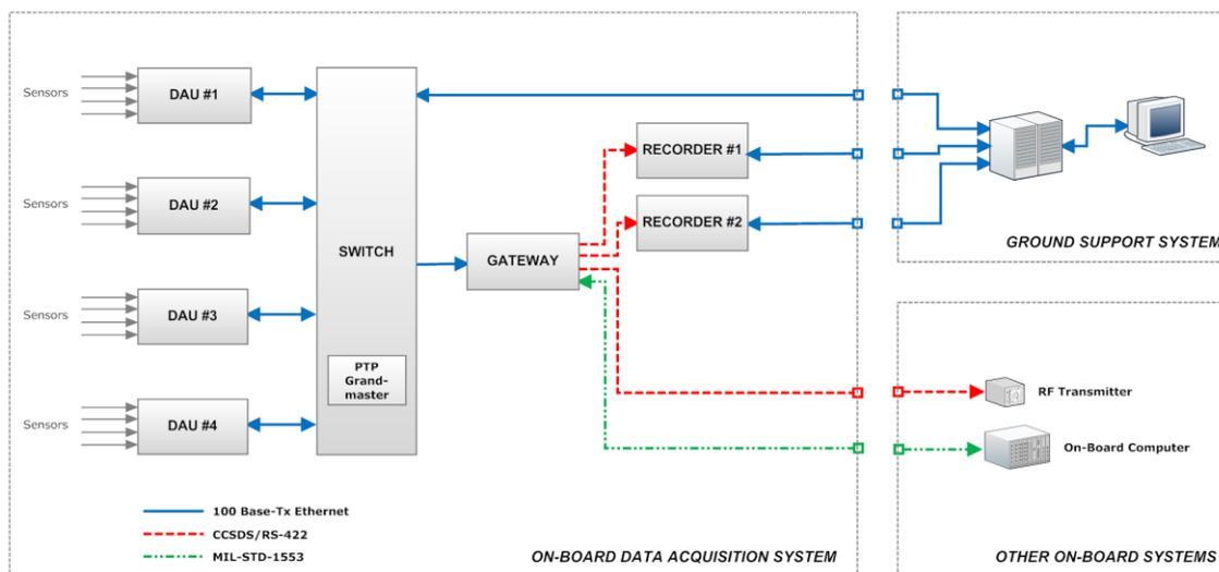
**Figure 3:** IXV Data Acquisition System
