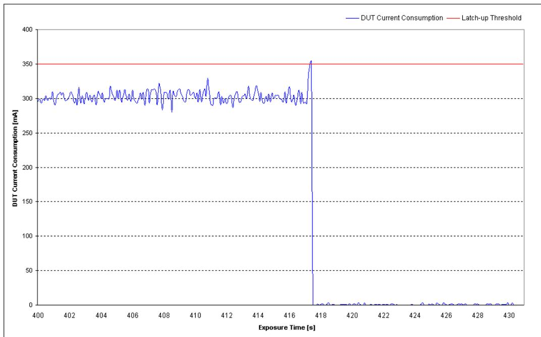
**Figure 6:** Current consumption during high-energy proton test
