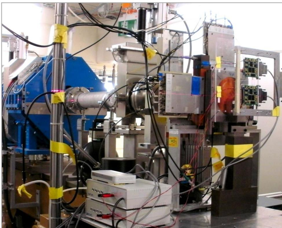
**Figure 5:** DAU controller module in the front of high-energy proton beam
