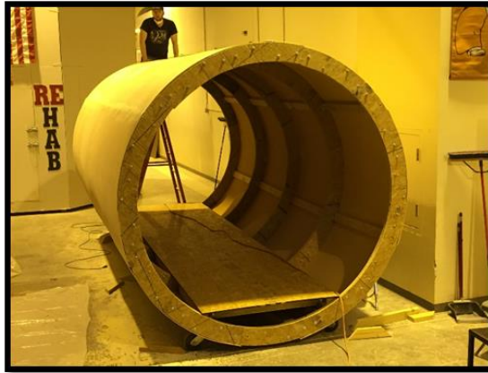
Figure 16: OSU's X-Hab team in the process of building a full-scale analog of an OASIS Greenwing
