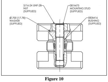
Section View of Model 261A03 ICP® 3-component Force Link
