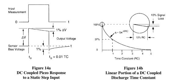
For example, when a 1,000 lb. static load is applied to a DC coupled force sensor that has a 2,000 second system DTC, within the first 20 seconds (1% of 2,000) the force output signal would decay 1%, or less than 10 lbs. So for 1% accuracy, the reading must be taken in 1% of the DTC, or 20 seconds. The entire system must be DC coupled, both signal conditioner and readout device, which means the sensor has a long DTC.
