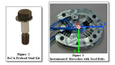
Also of importance, in preload and subsequent calibration, is the method in which the threads couple to the unit under test. Preload studs in adaptor rings or flight hardware bolts are usually used in a manner where the plate on top of the 3-component force ring has a clearance hole which the stud or bolt passes through. In the installation shown in Figure 4, the stud or bolt is not directly connected to the top plate by its threads; therefore it does not shunt any force.
