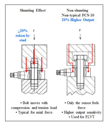
Figure 4 Preload Stud Thread Engagement Examples
