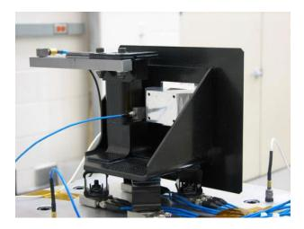
Figure 5 James Webb Space Telescope NIRSpec Bracket Assembly
