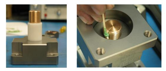
Figure 11 Preload Stud/Pilot Bushing Installation (Left), Thread Locker (Right)
