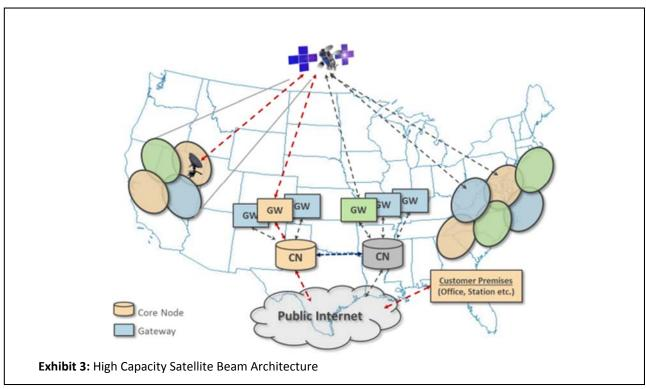
The spot beams concentrate the electromagnetic energy into a smaller area than conventional satellites, making the spot beams "hotter" than a wider conventional satellite beam. With an HCS end-to-end network, there have been three primary techniques employed to minimize and resolve EMI challenges:
