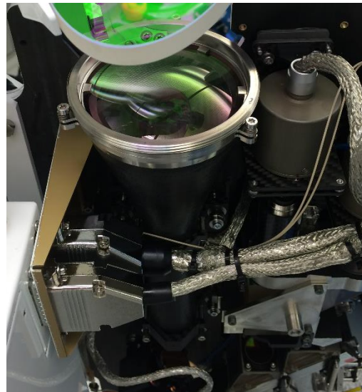
Exhibit 4: Laser communication terminal after final assembly and testing in ViaLight's facilities.
