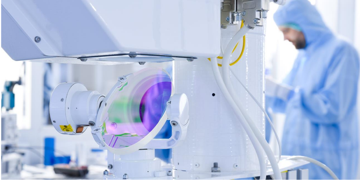
Exhibit 1: Stratospheric inter-platform LCT. Left: Coarse pointing assembly with entry aperture during integration in the clean room.
