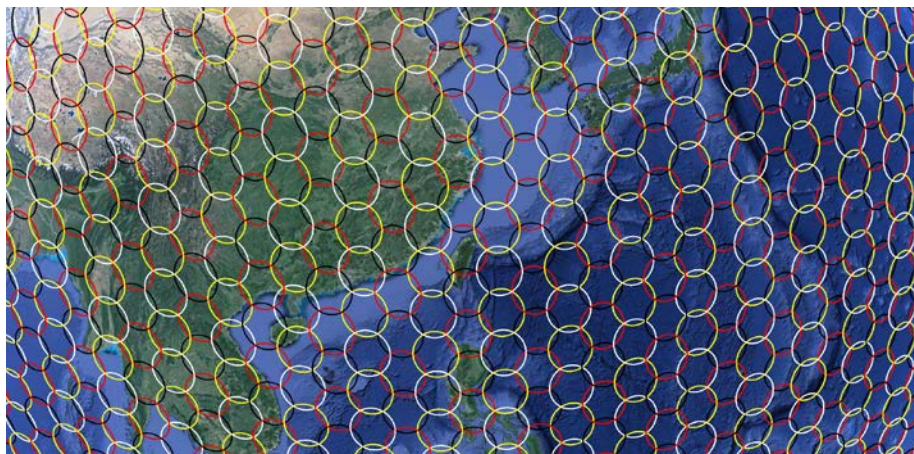
Exhibit 6: Grid-of-Beams – A notional 4-color reuse pattern over a large geographic area. Note that even though same colored beams are never adjacent to one another, there are many same-colored beams (interferers) nearby.
