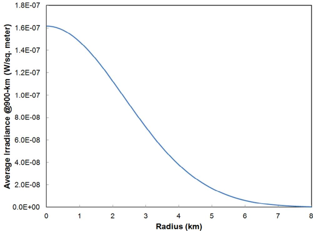
**Figure 5:** Average irradiance at 900-km range as a function of radius from the beam centerline for a 0.35-degree FWHM beam width.
