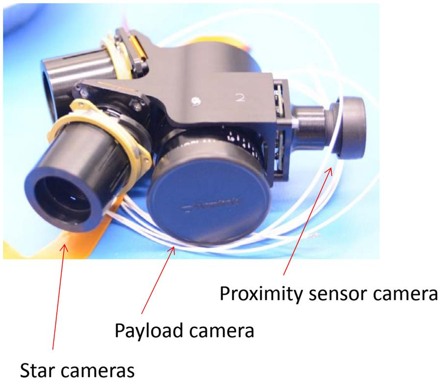
**Figure 6:** Photograph of the OCSat camera package including two star cameras, one flight camera, and one proximity camera.
