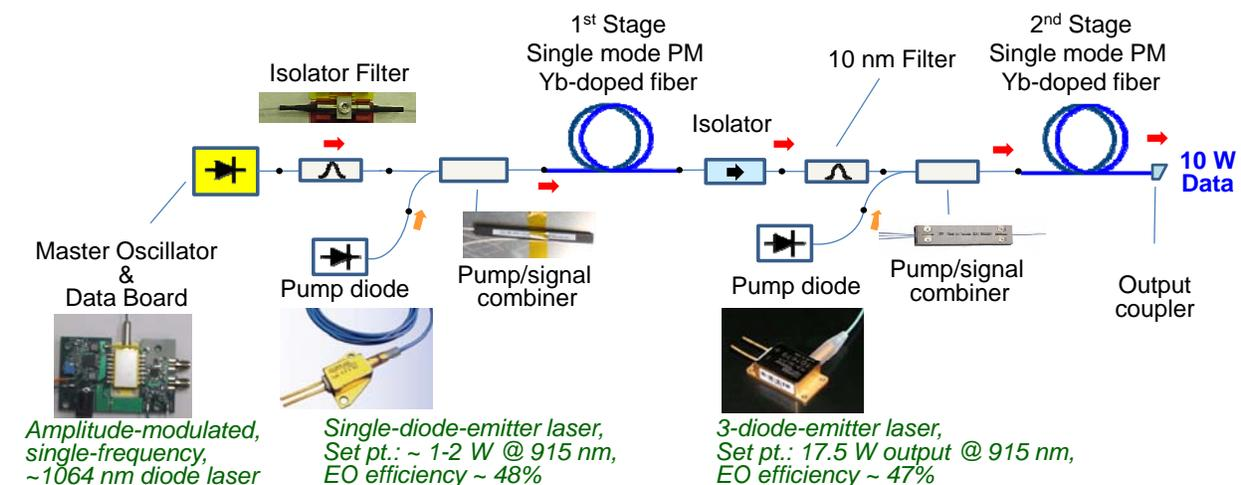
**Figure 3:** Schematic of the laser downlink transmitter.
