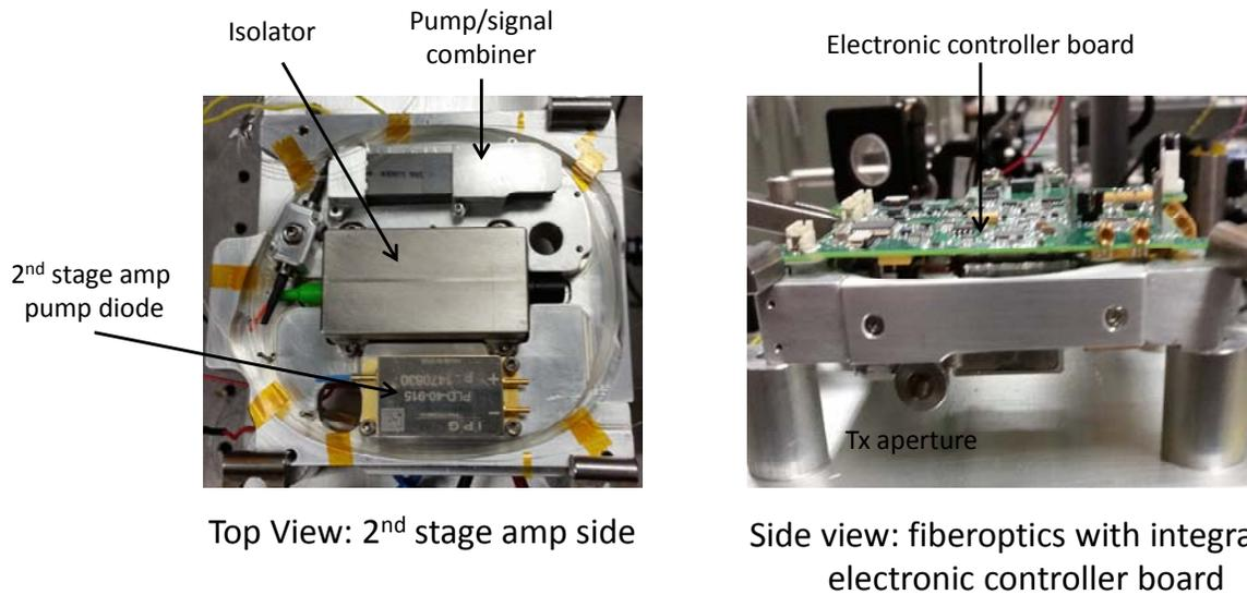
**Figure 4:** Photographs of laser transmitter.
