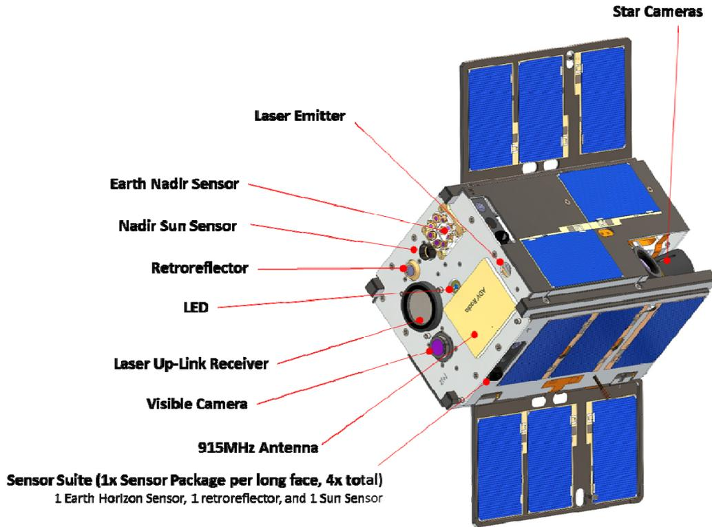
Figure 1: Rendering of the OCSD CubeSat.
