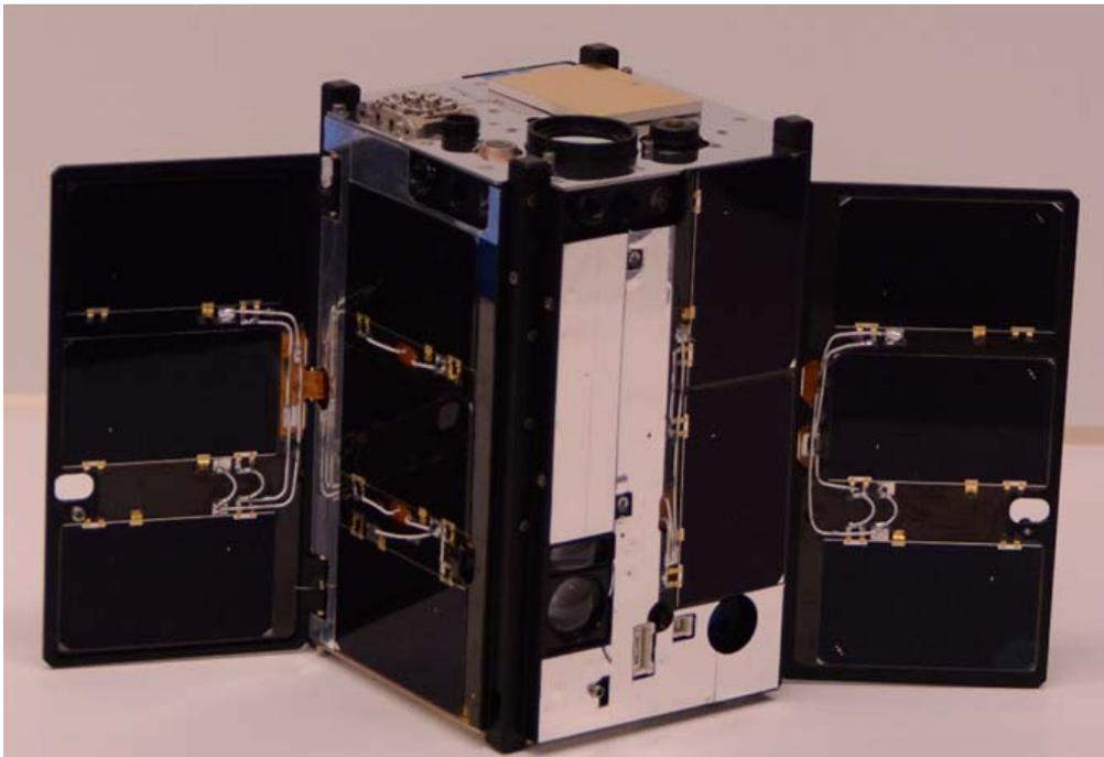
Figure 2: Photograph of the first OCSD CubeSat.
