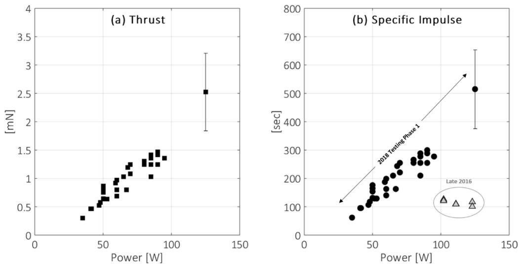
Figure 3: (a) The RFT-2 thrust measurements versus power and (b) measured specific impulse versus RF power between 40 W and 125 W at 0.5 mg/sec xenon mass flow rate. Data in gray show the previously presented results of The RFT-0 proof-of-concept system [5].
