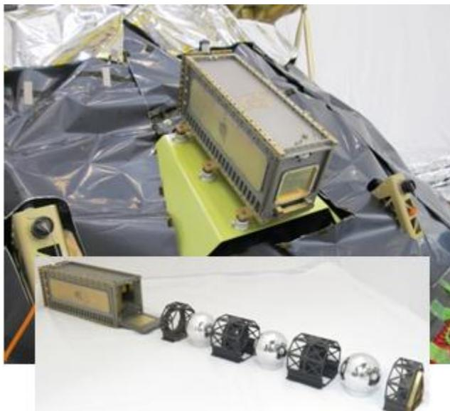
Exhibit 5: The Polar Orbiting Passive Atmospheric Calibration Sphere (POPACS) mission integrated to the final stage of the Falcon 9 Launch vehicle \*\*
