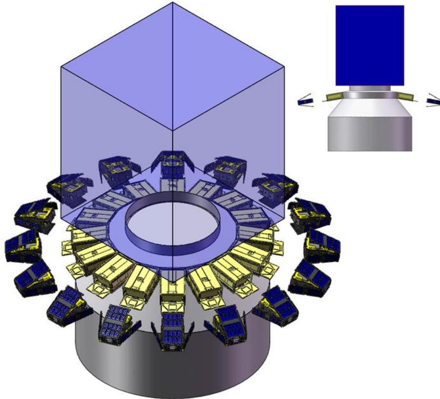
Exhibit 11: Sixteen 6U dispensers mounted underneath primary Payload. Thus an entire constellation may be deployed as a secondary payload.
