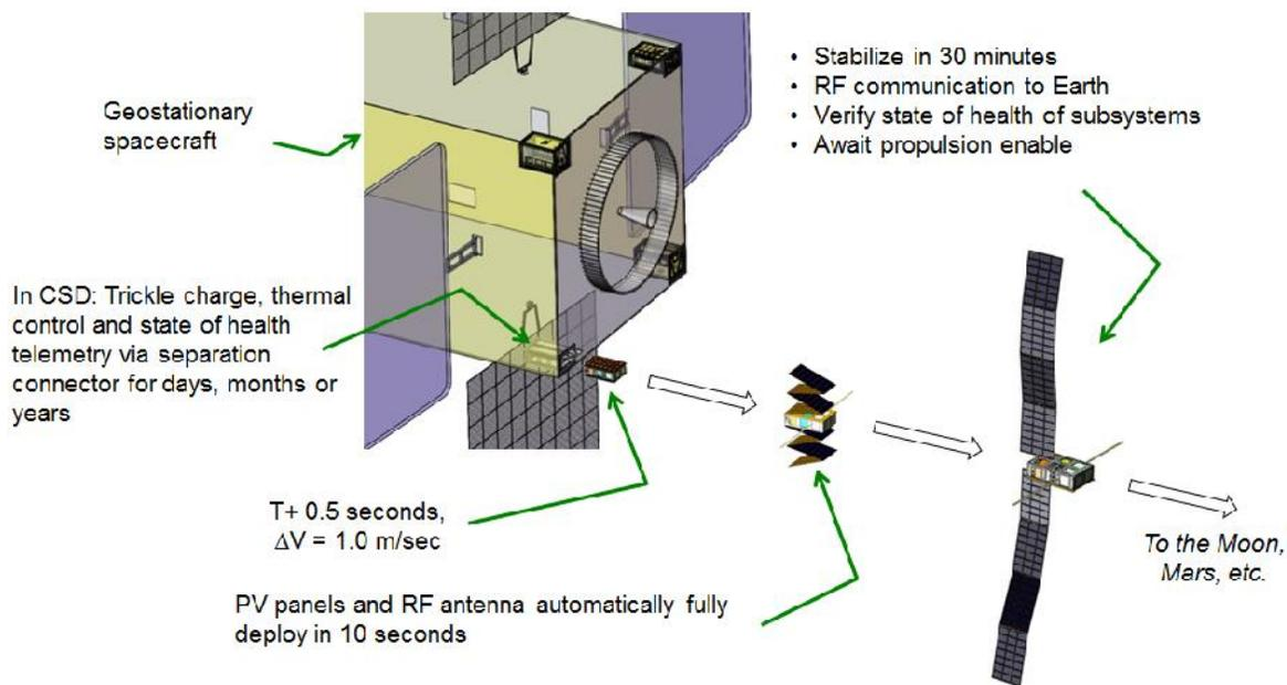
Exhibit 6: Hosting and dispensing the Lunar Water and Detection (LWaDi) from a geostationary spacecraft<sup>††</sup>
