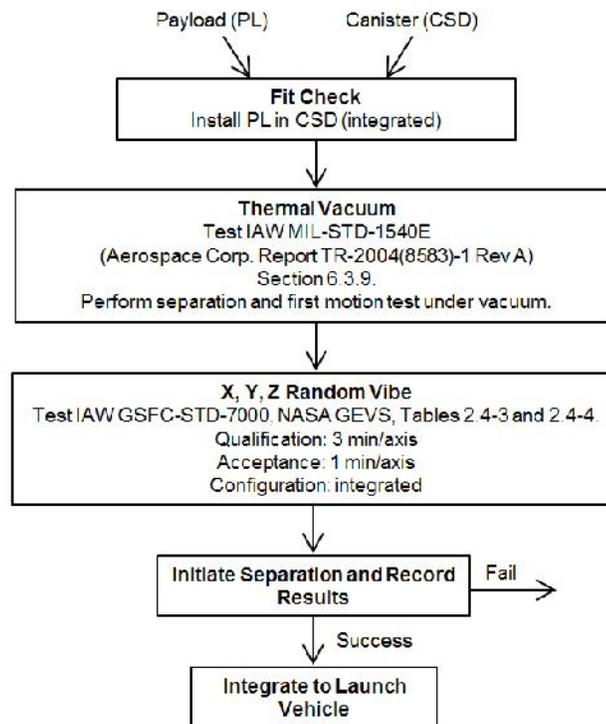
Exhibit 22: Test flow and requirements for payload
