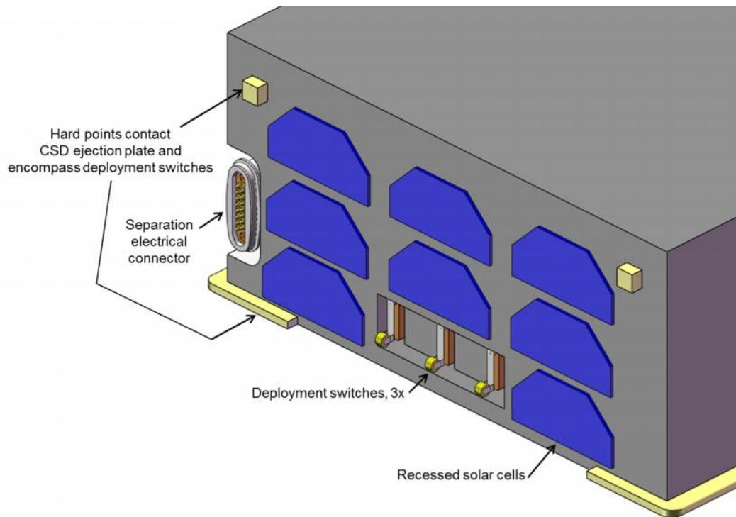
Exhibit 19: The ejector plate side of the payload showing the separation connector and three limit (deployment) switches
