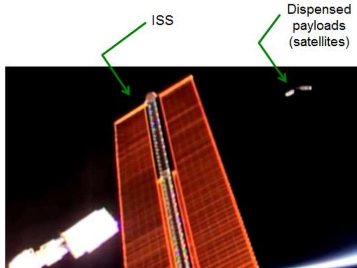
Exhibit 4: Two 3U Planet Lab's Cubesats (hosted payload) being dispensed from the ISS, the hoster of the payload
